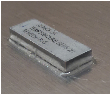
RFM3250 sensor epoxied with clear Gorilla Epoxy around the edges.
